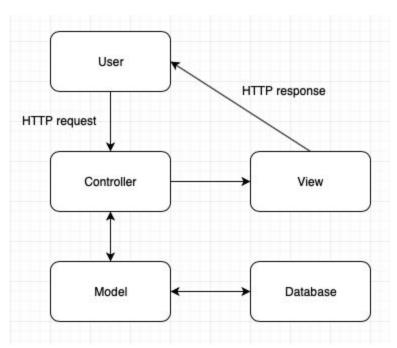
Model-view-controller (MVC) is a modern architectural pattern that divides the project into three interconnected parts. MVC allows for efficient code reuse and parallel development. This design pattern can possibly benefit the team.
